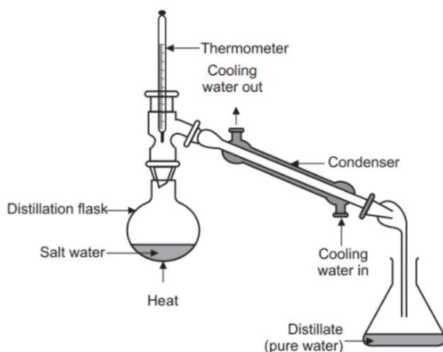
Note: separates mixtures by selective evaporation and condensation
